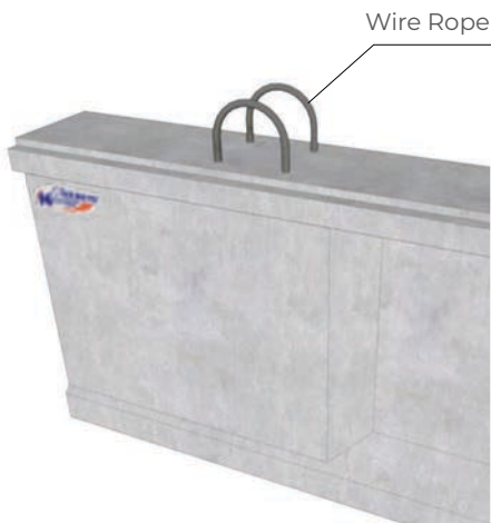
Alt. 1 Shear Key (Match Casting)
