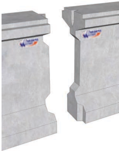
Alt. 1 Shear Key (Match Casting)
